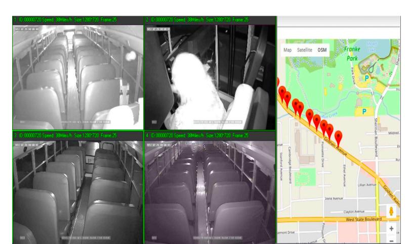
SD4HW Night Vision IR LEDs active for recording in total darkness, OSM map setting GPS breadcrumbs showing route SD4HW High Definition Road Facing camera, with IR LEDs disabled to prevent "ghosting" glare off windshield
