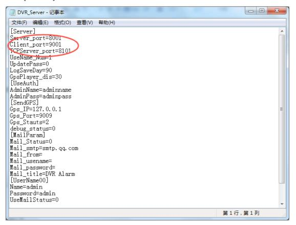
Noted: If the three ports have been used for other things, you just need to change the ports, like 7001, 6001, 6101 and then open 7001,6001,6101 three ports on your router, it will be ok. Also, all the server management will go on in the configuration file.
