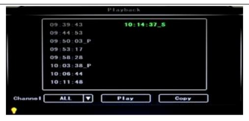
There are video date in the menu, it will display the vide time after enter the date, choose the playback time range as needed, press "Play" or click the interface "Playback "button to replay the video. Said is power outage file suffix "\_P", suffix "\_S" indicates an alarm trigger video files.
